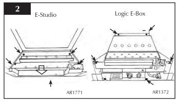
5.3 Decide on the retention method. If cable fixings are to be used remove the lower cover plate by unscrewing the three screws., Diagram 3.
